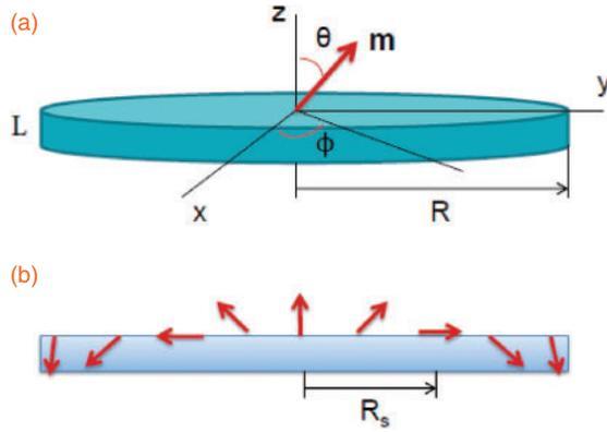
**Fig. 1.** Sketch of the cylindrical magnetic dot and the coordinate system used: (a)  $\mathbf{m}(\Theta, \Phi)$  is the unit magnetization vector described by the spherical polar angle  $\Theta$  and the azimuthal angle  $\Phi$ ; (b) Néel skyrmion magnetization distribution in the dot cross-section by the radial plane  $yz$ . The dot radius is  $R$ , and the skyrmion radius is  $R_s$ .
